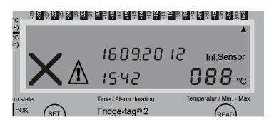
If the temperature and time conditions are outside the pre-set alarm parameters the following will be displayed on the screen:
