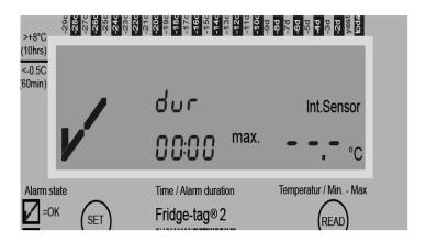
For a maximum of 1 minute no current temperature is displayed on the screen.
