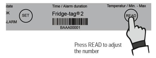
The SET button is used to save the number. After pressing the SET button the next digit will start flashing.
